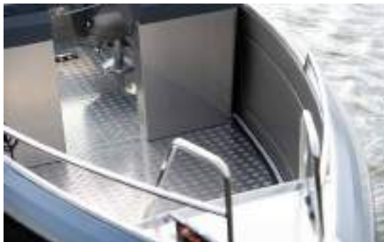
Durable and practical aluminium floor as standard
