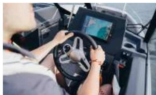
Buster Q 10" and hydraulic steering as standard
